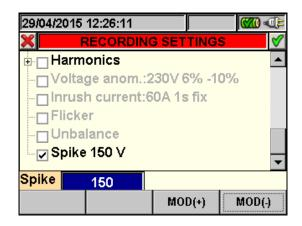
Fig. 97: Spike screen - setting control parameter
