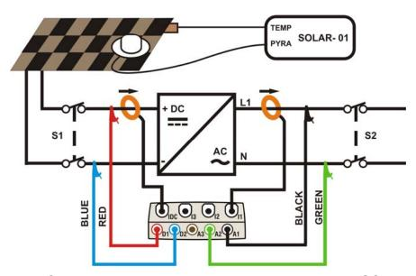
Fig. 159: Connecting the instrument in a PV-1 system with SOLAR-01
