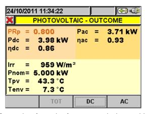
Fig. 138: Example of result of a test carried out with MPP300.
