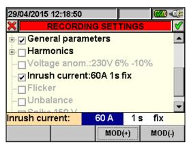
Fig. 92: Inrush current screen - setting control parameters
