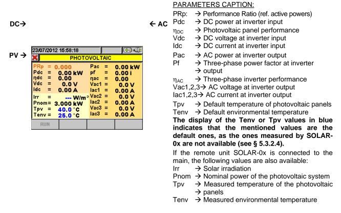
Fig. 20: Three-phase photovoltaic system page
