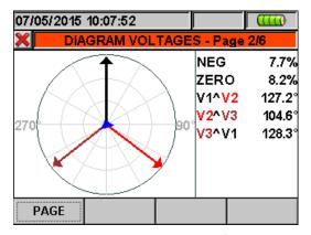
Fig. 48: Vectorial voltage diagram for 4-wire system
