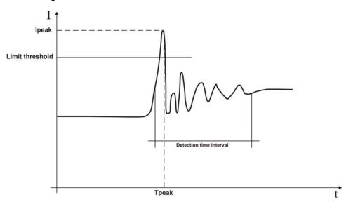
Fig. 175: Parameters of oscillating inrush current event
