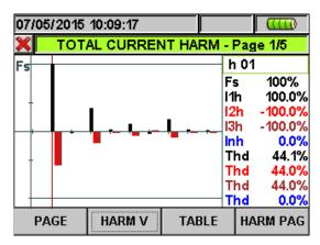
Fig. 42: Harmonic analysis of currents percentage/absolute for 4-wire systems
