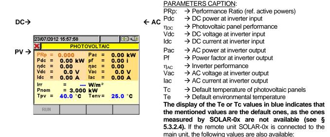
Fig. 19: Page of single-phase photovoltaic systems
