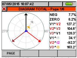
Fig. 47: Vectorial diagram total for 4-wire system
