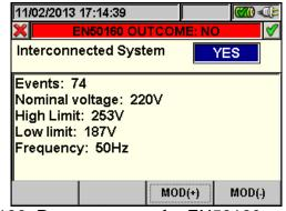
Fig. 130: Parameters set for EN50160 analysis
