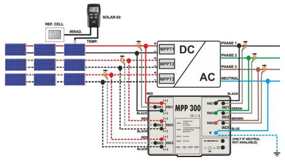
Fig. 164: Connection of MPP300 for testing a three-phase PV system
