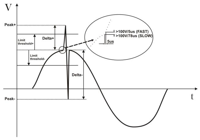
Fig. 177: Typical voltage spikes at 50Hz frequency
