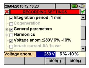
Fig. 90: Voltage Anomalies screen - setting control parameters
