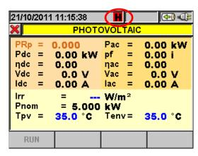
Fig. 4: HOLD function active at display
