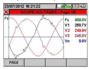
Fig. 145: Voltage scope in three-phase 4-wire system
