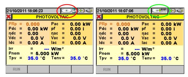
Fig. 101: Instrument in stand-by mode
