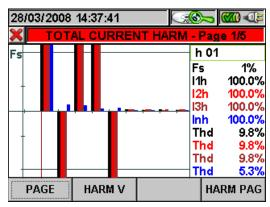
Fig. 146: Total harmonics in three-phase 4-wire system
