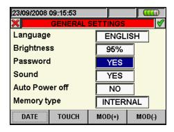
Fig. 12: Protection password settings screen
