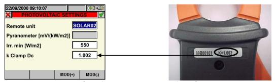
Fig. 67: Set of corrective constant for DC clamp
