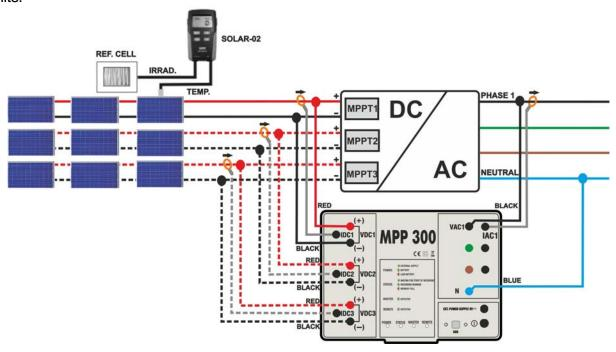
Fig. 163: Connection of MPP300 for testing a single-phase PV system
