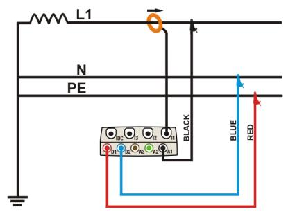
Fig. 165: Meter connection in a Single phase system
