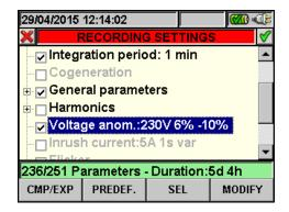
Fig. 89: Voltage Anomalies selection screen
