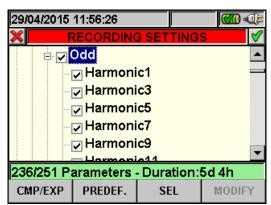
Fig. 86: Harmonics sub-levels: odd harmonics selection
