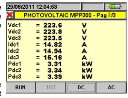
Example of a DC screen for PV systems with 3 MPPTs
