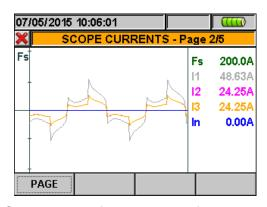
Fig. 37: Current waveforms screen for 4-wire systems
