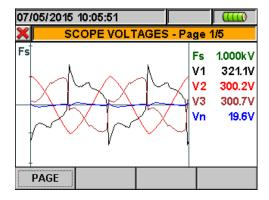
Fig. 36: Voltage waveforms screen for 4-wire systems
