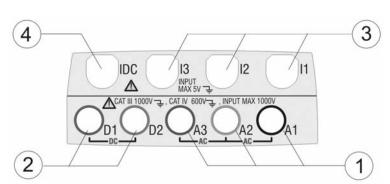
Fig. 1: Description of meter's front panel
