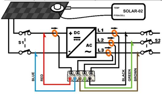
Fig. 162: Connecting the instrument to a PV-3 system with SOLAR-02
