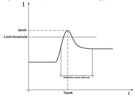
Fig. 174: Parameters of standard inrush current event
