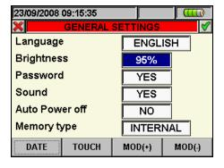
Fig. 11: Adjust brightness screen
