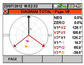
Fig. 147: Total vector diagram in three-phase 4-wire system
