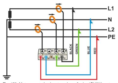
Fig. 173: Meter connection in a two phase 3-wire 1PH3W system
