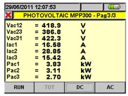
Example of an AC screen for PV
