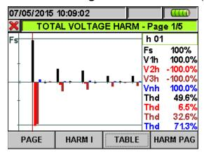
Fig. 41: Harmonic analysis of voltages in percentage value for 4-wire systems In all case the full scale of graphs is automatically set from meter depending on measured values.
