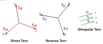
Fig. 176: Decomposition of a vectors tern
