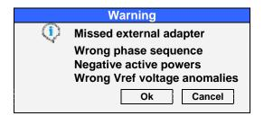
Fig. 108: Warning message errors screen
